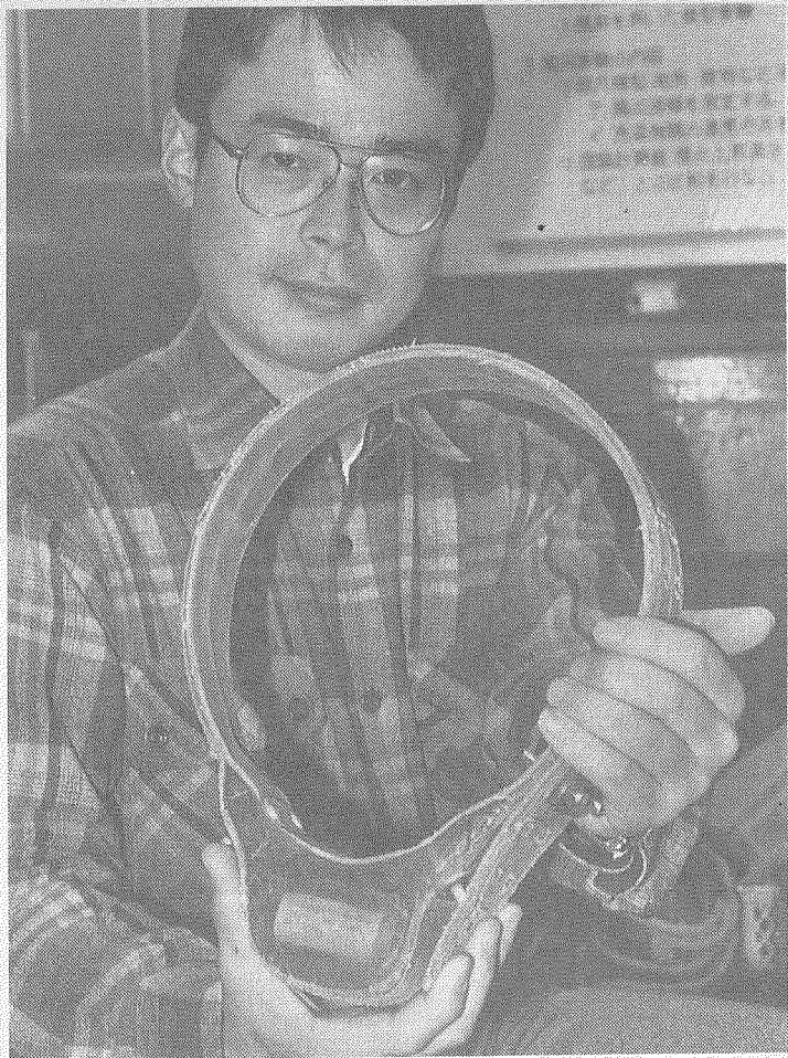
A SPECIAL COLLAR for brown bears, fitted with a transmitter, will be used in an ecological study in Hokkaido. KYODO PHOTO
